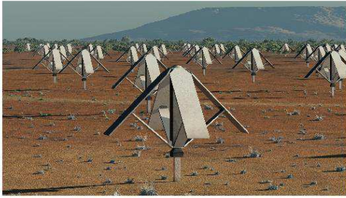
Figure 1: SKA sparse aperture array station of dipole elements for about 70–450 MHz. Graphics: Swinburne Astronomy Productions and SKA Project Office (SPO).
