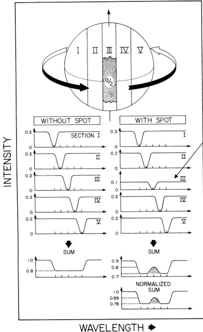
As a spot moves across the star the line profile changes. From an observed line profile, one can construct an image of the surface of the star. This technique has been applied to many different types of stars.
