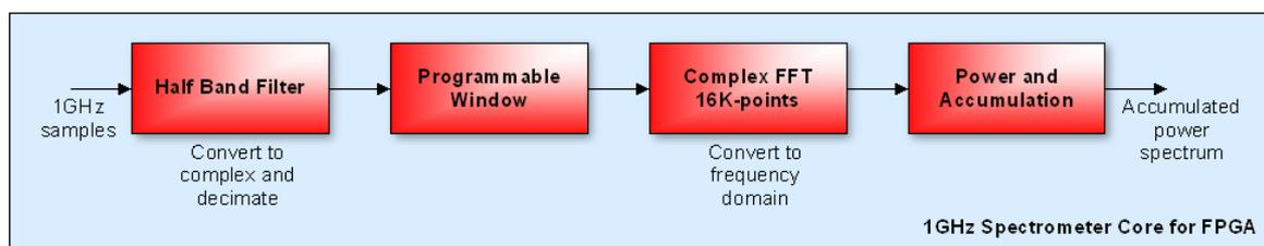
**A block diagram of RF Engines 1GHz Spectrometer Core for FPGA**
