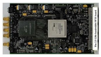
Fig. 7 Currently in development: The 2.5 GHz bandwidth FFTS. The board makes use of a first sample of E2V's 5 GS/s 8-bit ADC.
