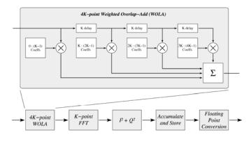
Fig. 5 Block diagram of the polyphase signal processing pipeline.
