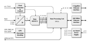
Fig. 2 Block diagram of the new MPIfR 1.5 GHz digitizer/analyzer board. The board can be equipped with a single- or dual-input ADC (ADC083000 or ADC08D1500). The optional GigaBit Ethernet interface allows high speed data acquisition with transfer rates up to 85 MBytes/s, which are required for pulsar or transient searches.
