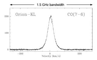
Fig. 4 First light spectrum of the new MPIfR-based 1.5 GHz bandwidth FFTS board towards the hot core Orion-KL. The high-excitation CO(7-6) transition at 806 GHz was observed with the central pixel of the CHAMP<sup>+</sup> array at APEX (24. October 2007).
