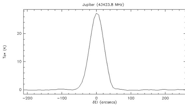
Figure 5. Total power (512 MHz) elevation pointing drift obtained from a scan on Jupiter at 43 GHz .
