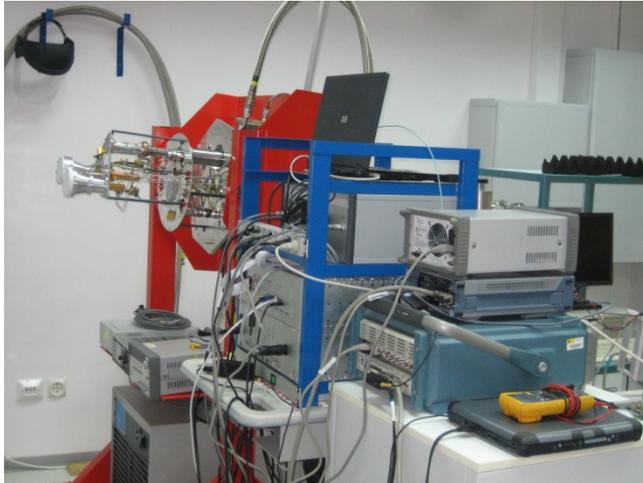
Figure 4. Photograph of the QuiK cryostat of the Yebes 40-meter radiotelescope, with 22 and 43 GHz horns visible.
