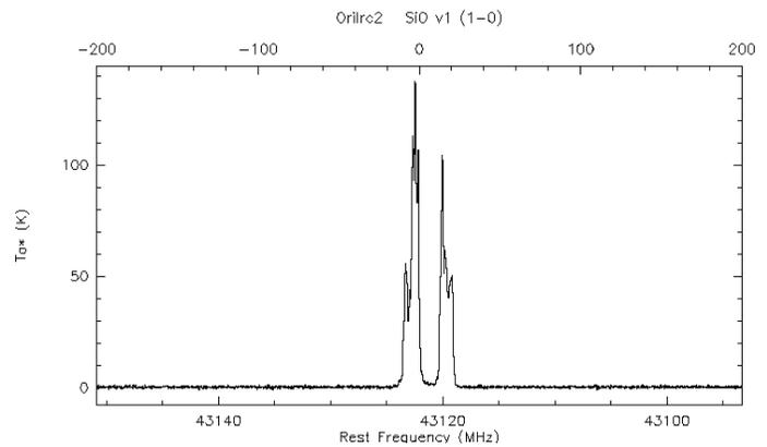
Figure 6. Spectrum of the SiO 1-0  $v=1$  maser towards Orilrc2 obtained with the new Q-band system over a total integration time of 30 seconds.
