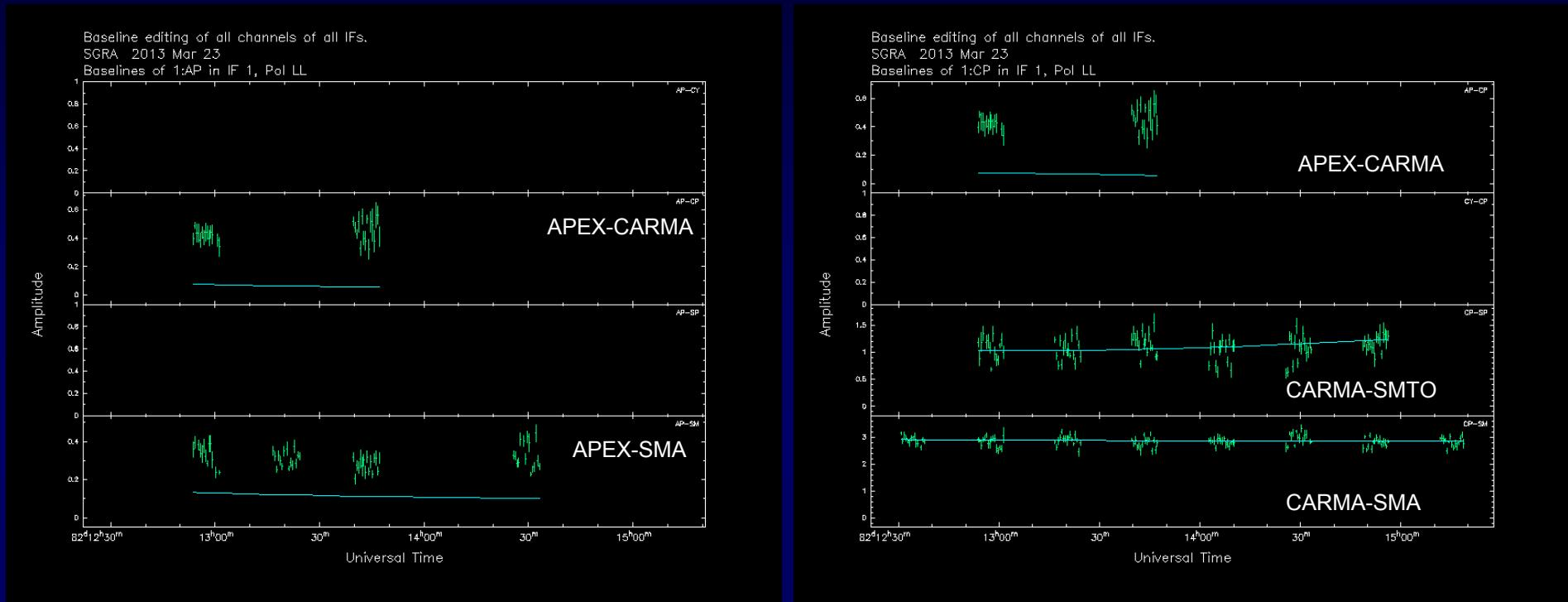
The correlated flux measured on APEX baselines is about a factor of 2-4 higher than expected for a circular Gaussian source of 37  $\mu$ as FWHM.
