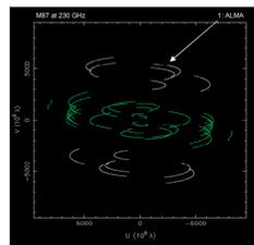
The uv-coverage for a mm-VLBI experiment on M87 at 230 GHz with the following stations: IRAM-30m, IRAM-interferometer, HHSMT, eSMA (SMA + JCMT + CSO), CARMA, LMT and one station in Chile (APEX/ASTE first, ALMA after 2012).
