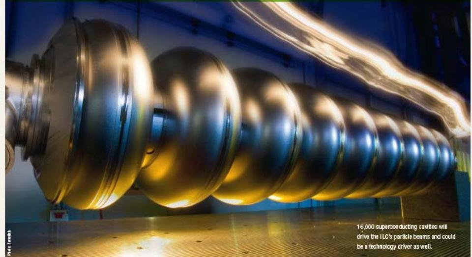
16,000 superconducting cavities will drive the ILC's particle beams and could be a technology driver as well.
