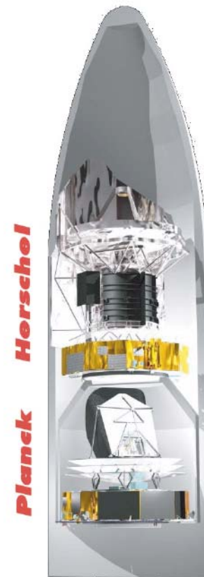
FIG 1.11.— Planck and Herschel ready for launch under the Ariane 5 fairing. The two satellites separate just after launch and proceed independently to their final orbits. View courtesy of Alcatel Space (Cannes).
