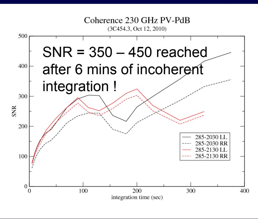
good VLBI-phasing efficiency of the 6 elements of the PdB interferometer
