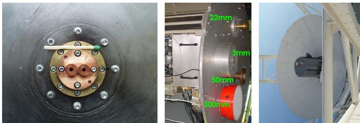
*Fig 2: Left: The tiny two horns of the 3 mm receiver and a match visualizing the scale. Center: The feeds of the four receivers, which are installed in the receiver multi-box II. Right: The receiver multi-box II shifted into the prime focus of the telescope, with the 6.5 m adaptive sub-reflector behind.*
