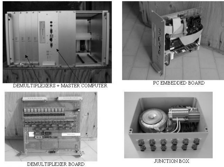
Fig. 2. Master computer/demux rack and junction box
