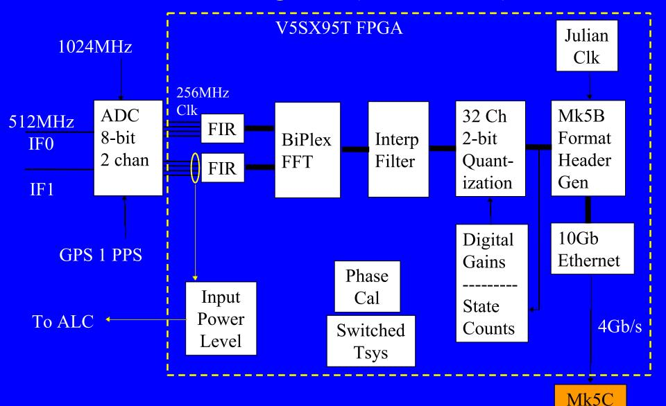
Each 512 MHz IF split into 16 channels, each 32 MHz.
