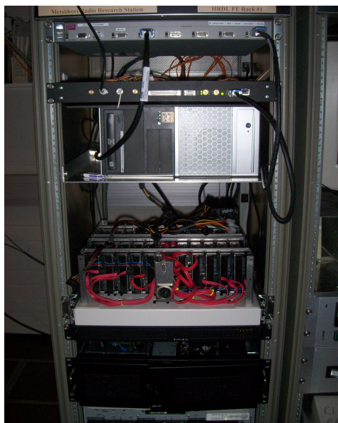
New VLBI rack with the 10 Gigabits internal switch, ibob, windows-ibob development pc, new host computer for the disk pack and the disk-pack itself.
