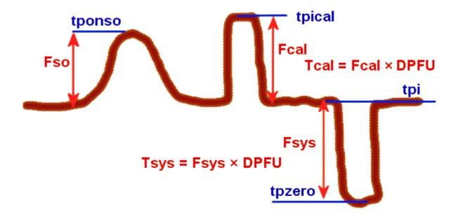
Source, cal signal and -20 dB levels Original FS readings are marked in blue
