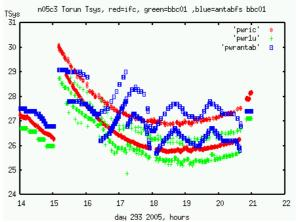
The high quality of the system is shown by the stability of the red curve from IF total power. The green curve shows reasonable accuracy, but the accuracy of the "tpdiffgain" method is obviously limited. However the 'pwrantab' curve is obviously incorrect, showing breaks in the curve where the BBC attenuator changes by 1 step, which suggests an interaction of straight-line fitting with the attenuator switching steps.
