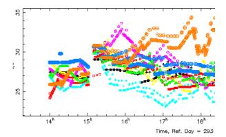
The individual channels on the antabfs plot show a seemingly random off-source noise level, increases of 1.5K in antenna temperature caused by 3C454.3 can be seen on top of this. To check this a simple script was used to plot power in IF channel "c", and in bbc01 which is connected to it, scaled according to the variable attenuator setting. The traces are pwric and pwr1u in the plot. The '1u' channel taken from the antabfs file is pwrantab.
