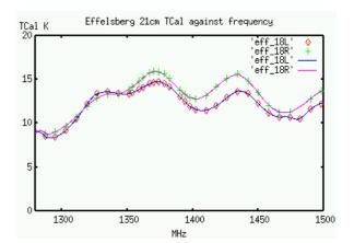
Points are measured every 8MHz. One sees a sinusoidal variation with a period of about 50MHz. The usual cause of ripples is mismatch in directional couplers used for putting in the cal. Also 18cm couplers are often not directional, but merely a probe in the waveguide. Then power is also sent out of the horn and returns as frequency - dependent reflection.
