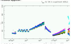
(n05L2 Onsala) Here large gradients appear because a straight-line fit is used between faulty Tsys points. So it is necessary to inspect all antabfs files at the stations, and hand-edit the logs if results like this appear.
