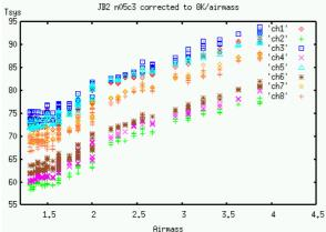
This looks more realistic. There are two families of curves corresponding to odd and even channels, L and R pol with different TRec, (only channel 8 is in the wrong group). So except for a scale factor, calibration according to airmass can give a useful method of checking calibration in individual channels.
