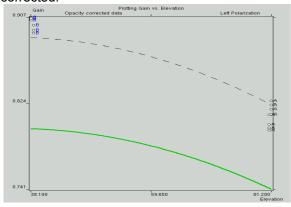
Note that to correct for opacity, values for Trec and spillover in the rxg files are needed (example in Appendix). An irritation is that the rxg files have two places for gain (LCP,RCP), but only one Trec. This should perhaps be changed since Trec is often different in two polarisation channels, but gain does not vary.
