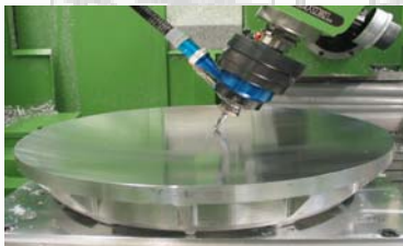
A 50 cm concave mirror being manufactured at MPIfR. The surface accuracy is 5 micron.
