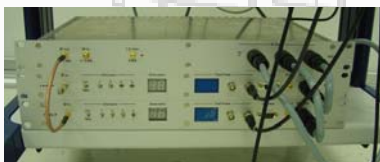
The IF-processor preparing the signal for the spectrometers
