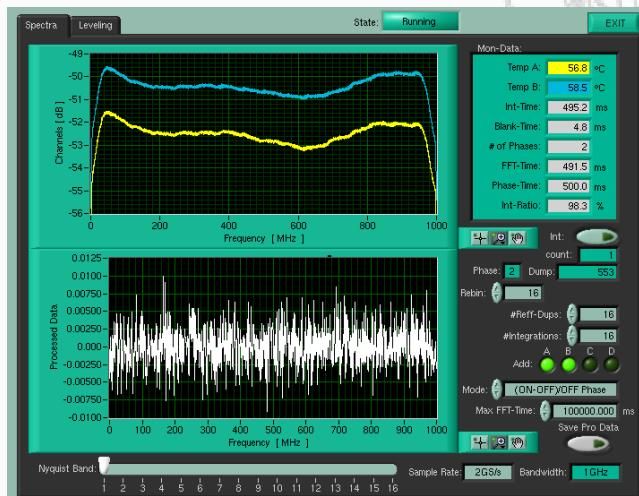
Screenshot of the user-friendly LabView-Interface to the APEX FFTS. This interface can be used for online data quality control as well as system debugging during installation phases of various receivers. – In the upper panel the two receiver-bandpasses are shown. In the lower panel a sky integration is displayed.
