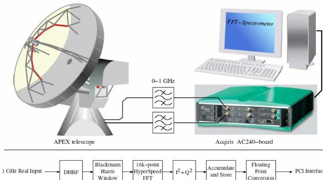
The APEX broadband FFTS is able to cover a frequency-bandwidth of up to 2x1 GHz using two commercially available ADC boards. - The lower flow illustrated the FPGA signal processing pipeline.
