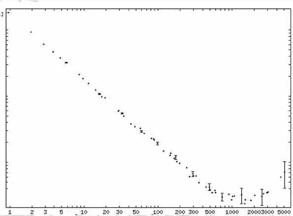
The measured Allan Variance of APEX FFTS shows extremely high stability resulting in possible integration times of more than 1000 seconds.
