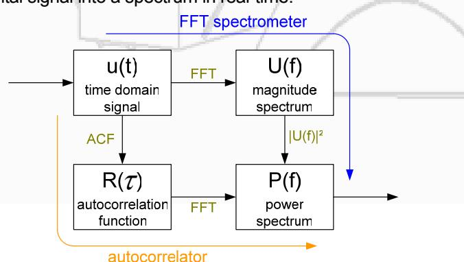
*"Wiener-Khinchin-Theorem": FFT spectrometer implement an alternative approach for obtaining the power spectrum of a given time signal.*
