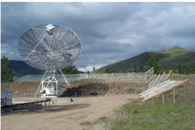
The “fences” near Antenna 1. These metal mesh screens shield the spillover lobes from the ground, giving a 2K improvement in system noise.
