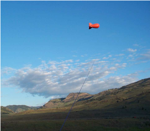
The aerostat in flight over the White Lake basin in May. Note one of the peripheral tethers rising from the foreground. The point at which the three peripheral tethers meet is approximately 200 m above the ground. The aerostat flies on a single tether above this point, with the length of that tether being one of the variables under test. At the time of this photo the tether length was 20 m. Experience quickly showed that longer is better, and the length now used is 150 m
