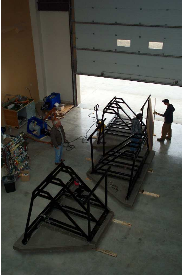
The large structure development area , a two-storey space at the east end of the building for working on mechanical aspects of projects such as the LAR. Shown are winch frames for the LAR project.
