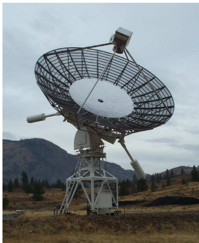
Antenna 7 of the Synthesis Telescope at DRAO, showing the aluminum tape covering the central portion, as described in the text.
