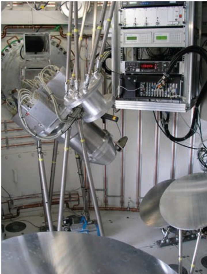
Figure 2: LABOCA in the Cassegrain cabin of the APEX telescope. The receiver is in the centre of the picture. Four of the five mirrors used for the optical coupling are visible.
